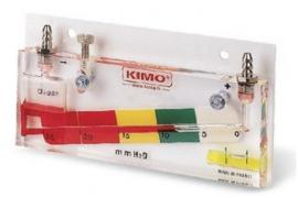
If the **RED** Liquid moves into the **RED** Zone you must change the filters immediately (see previous page on how to change filters).
